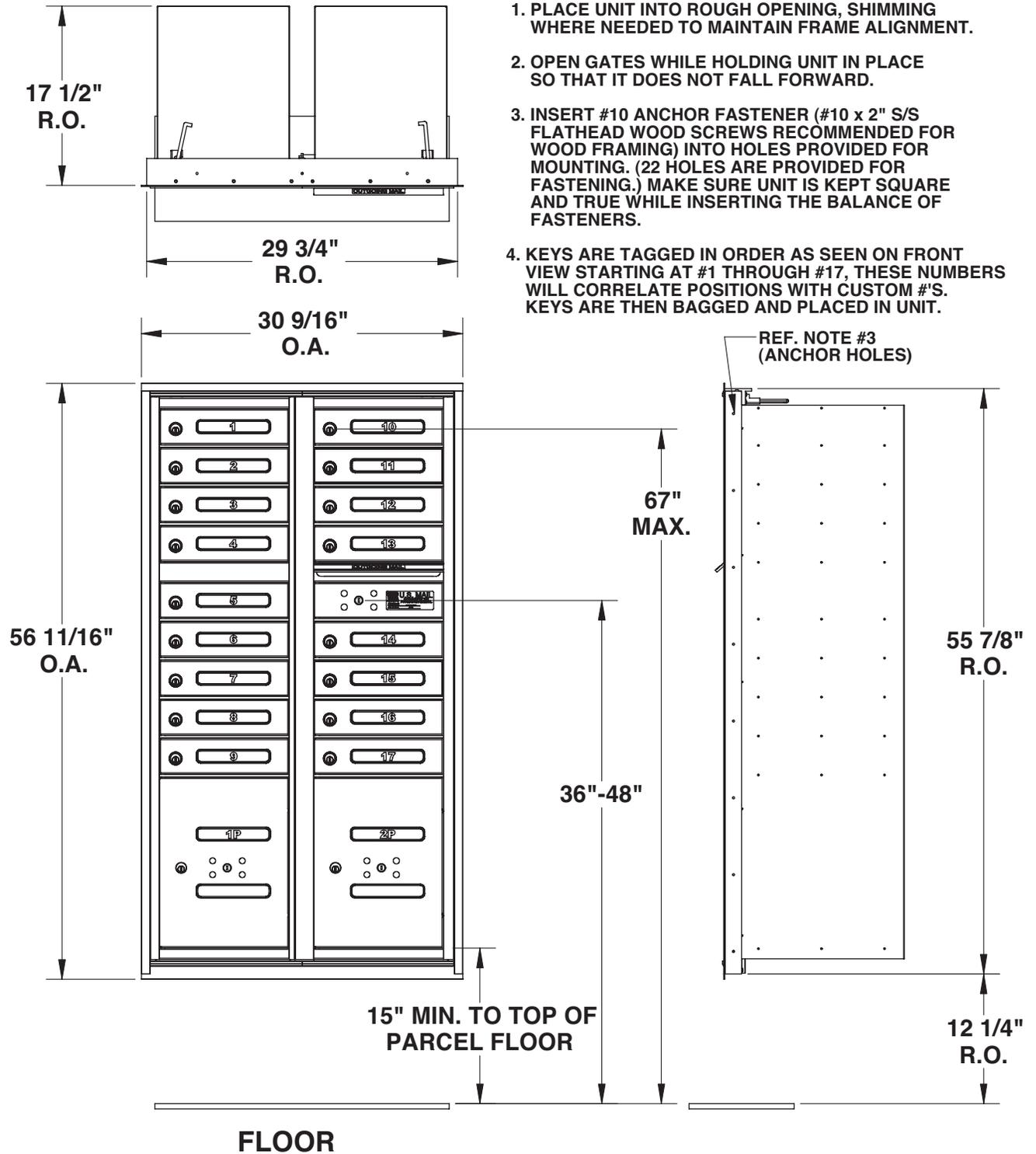
1. PLACE UNIT INTO ROUGH OPENING, SHIMMING WHERE NEEDED TO MAINTAIN FRAME ALIGNMENT.
